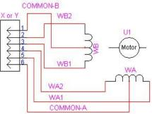
Typical Bipolar Motor Connection To the BiStepA05 Board
