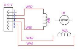
Typical Bipolar Motor Connection To the BiStepA05 Board
